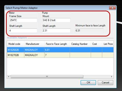
Select Pump/Motor Adaptor based on Pump and Motor properties
